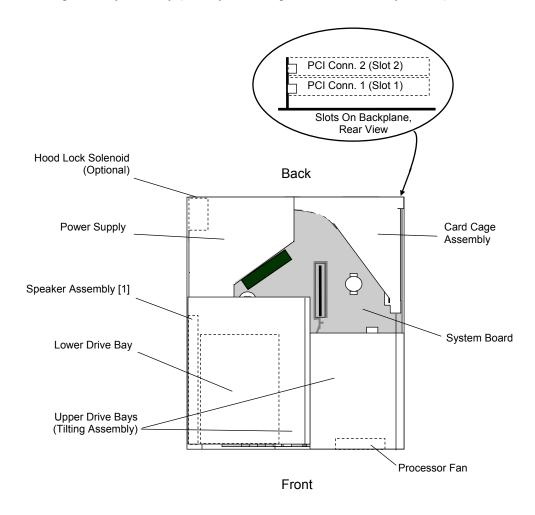
Figure 2–4. Small Form Factor Chassis Layout, Top View
